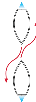
Head on situation – both alter course to starboard and give way to the other vessel.
