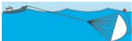
SEA ANCHOR – A small drogue acting like a parachute, dramatically slows the rate of drift.
