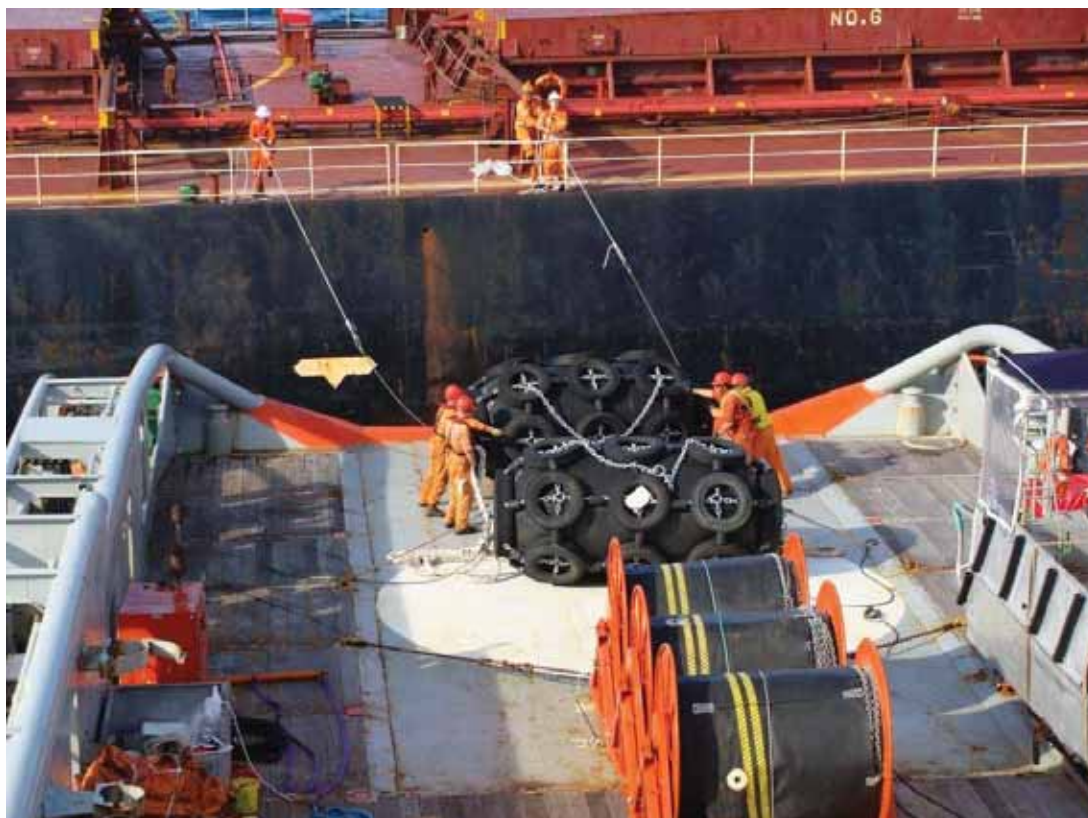
Maritime Safety Queensland officers and the National Response Team used oil booms to trap and contain any fuel oil lost during the oil recovery from the Shen Neng 1 in 2010. Maritime Safety Queensland values the professionalism, integrity and welfare of our staff.
