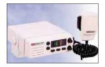
2. 27MHz – these are relatively cheap, easy to operate transceivers and are common in small boats. Their range is essentially 'line-of-sight' and they may be subject to interference noise.
