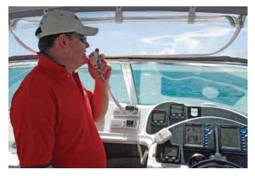
A marine radio transceiver is a vital safety aid, especially for boats travelling offshore. It provides a means of advising marine rescue groups of your itinerary and keeping in contact with them and other boats nearby, checking the weather and receiving navigational warnings. In an emergency, marine radio is your best means of summoning help.
