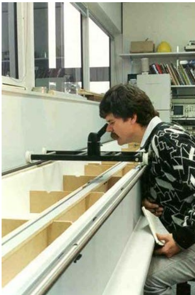
Figure 10 - Calibrating an Aquatrak sensor in a calibration rig.
