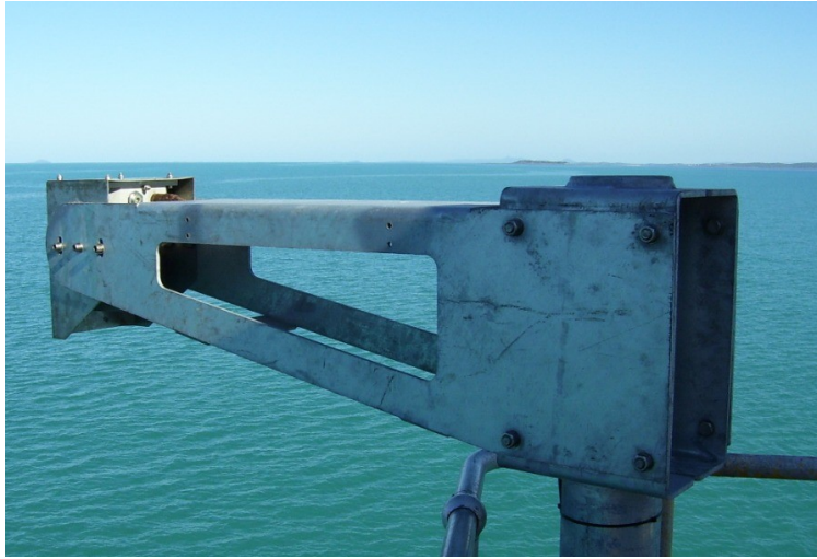
Figure 6 - Laser wave ranging gauge in operation at Hay Point.
