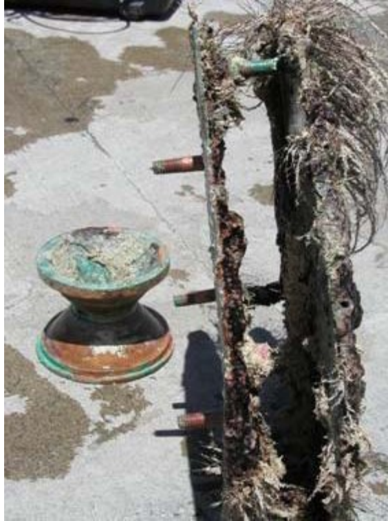
Figure 11 - Biological fouling is a real problem, especially in near shore tropical waters.
